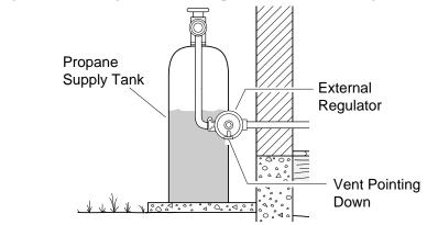
Figure 13 - External Regulator With Vent Pointing Down
